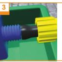
Remove collar. Push 6mm pipe through collar and attach to AQUAvalve nozzle Rescrew collar - DON'T overturn... when you
